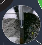
Unrecyclable materials are processed into fuel, which has a similar calorific value to brown coal. The fuel actually consists of parts of unprocessed waste.
