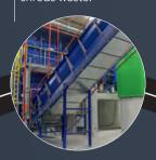
Shredded waste proceeds into a sieve that separates it according to size.
